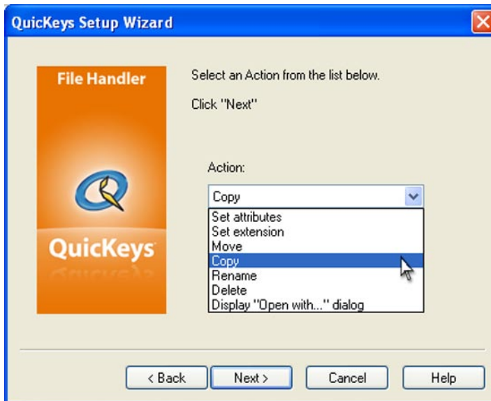
Figure 7-2: This dialog appears when you click the File Handler button in the Setup Wizards view and choose to create or edit a File Handler Action.
