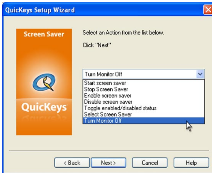
Figure 9-2: The Screen Saver Action lets you change screen savers, turn your screen saver on and off, and sleep your monitor with the tap of a key.
