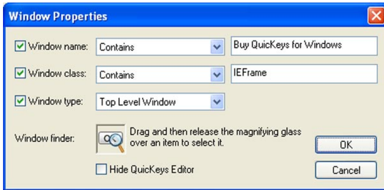
Figure 12-6: The Window Properties dialog tells QuickKeys the specifics of the window it should be looking for. Just drag the Window finder tool onto the desired window to auto-populate the fields with its defining characteristics.
