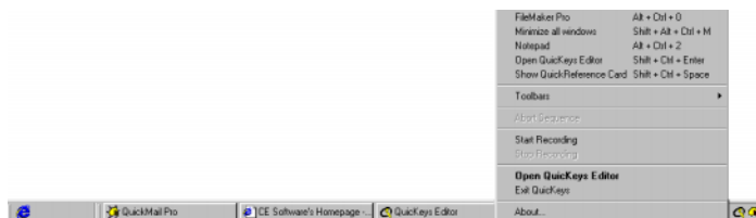
FIGURE 1: By default, you can open the QuicKeys menu from the Windows taskbar. The QuicKeys menu is located in the status area of the taskbar.
